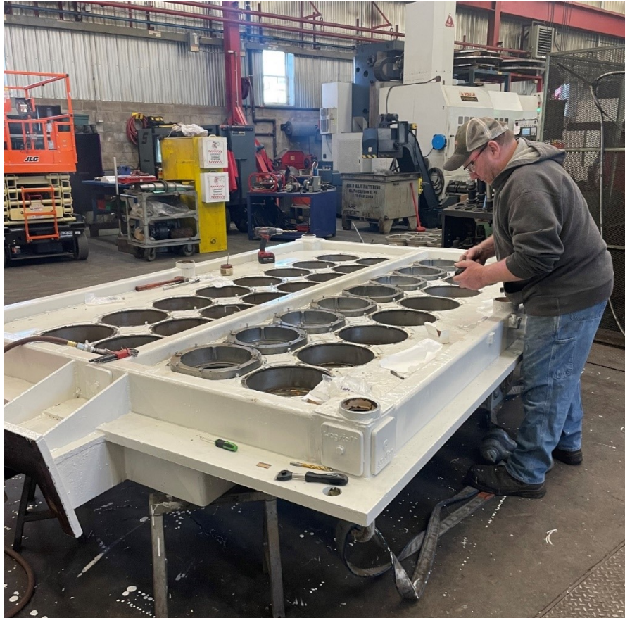
Figure 16. Wise Chem E-212-F coated on a vertical direct chill casting table.
