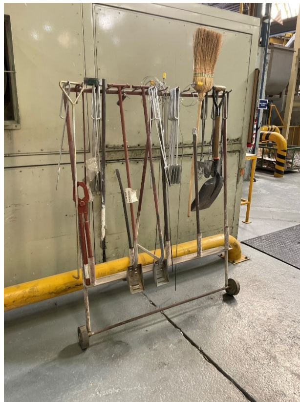
Figure 12. Example of how to properly store molten metal hand tools.
